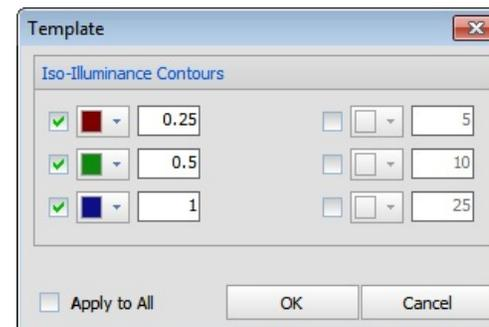
Selecting the "Apply to All" checkbox will associate the chosen values and colors to **Templates** for all **Luminaire Types** in the **Luminaire Schedule** regardless of what is in the **Active Item** selection set.
