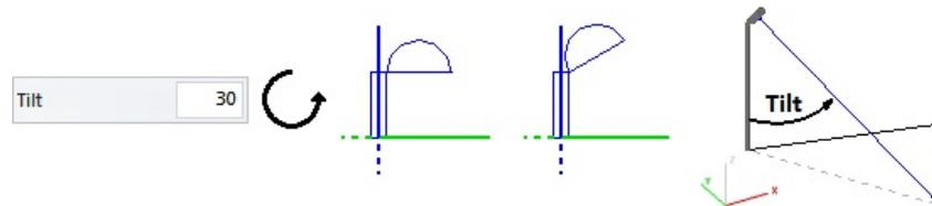
This command is useful with odd-angled alignments necessary in site lighting, as shown at right where the angle is specified by using **Object Snap** to align to the parking lot line.
