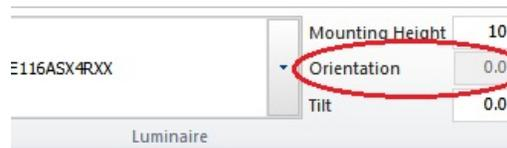
**Tilt** is the rotation angle applied in the vertical **plane**. Unlike **Orientation**, **Tilt** angle is applied **in place** of the angle used to define the **Luminaire Symbol** in the **Luminaire Editor**. Angles are applied in a counterclockwise fashion when viewed from the **East Elevation**, with 0° being straight down; thus a positive tilt angle rotates the **luminaire** up as would be expected.
