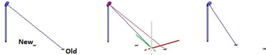
**Aim to Surface** (found on the **Luminaire tab**) is applicable to the **Reaim** command just as it would be to the initial **Place and Aim** command. Visual can determine when the mouse is placed "over" a **Solid Object** and the **Active Plane** can be automatically and temporarily changed to the **plane** of that **Solid Object** such that when the mouse is clicked the aiming point is placed in the **plane** of that **Solid Object**.
