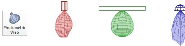
Analogous to the **Photometric Web** button when inserting **Luminaires**, the **Distribution** button found on the **Luminaire** tab of the **Ribbonbar** initiates a *drop-down menu* that allows the user to turn on or off **Photometric Webs** in the **Design Environment** for all **Luminaires**.
