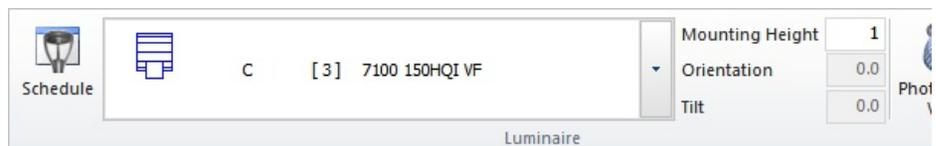
After a **Luminaire** is inserted with **Place and Aim**, Visual continues the command to allow for multiple insertions. To end the command, right-click or press **Enter**.
