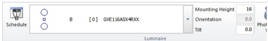
After a **Luminaire** is inserted with **Place and Orient**, Visual continues the command to allow for multiple insertions. To end the command, right-click or press **Enter**.
