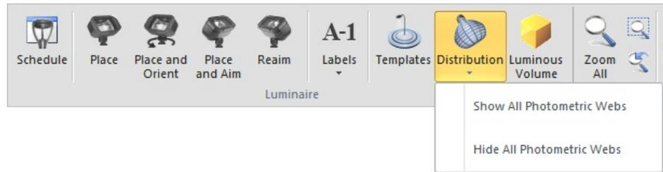
The **Luminous Volume** button directs Visual to display the luminous dimensions graphically (as seen in the wireframe view at middle-right) for each placed **Luminaire** in the **Design Environment** in conjunction with the **Symbol** as defined in the [Luminaire Schedule](#).
