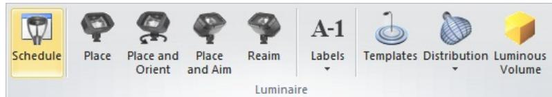
To **Place and Orient** a **Luminaire**, select a **Luminaire** from the **Luminaire Type List** then select the **coordinates** desired for the location of the **Luminaire** with the mouse, keyboard entry or **Object Snap**. Secondly, specify the **Orientation** with the mouse, keyboard, or **Object Snap**. Visual displays the angular change as the mouse is moved to illustrate the end result.
