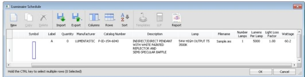
A default **Symbol** will be created for the new item based on the luminous opening dimensions included in the *photometric file* and not the physical dimensions of the entire *luminaire*. The *symbol* dimensions can be modified if necessary; see [The Symbol Editor](#).
