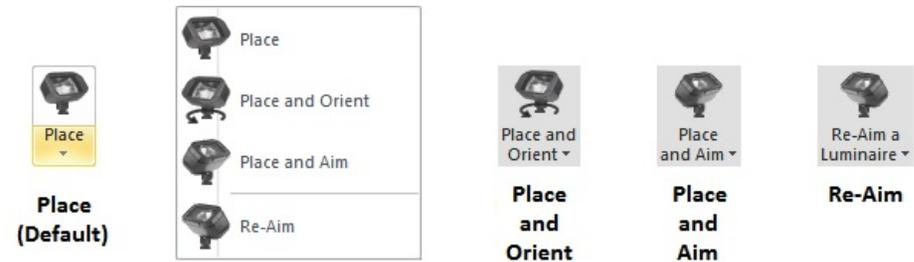
To **Reaim a Luminaire**, left-click the **luminaire Symbol** or the **Aiming Line** (if displayed). Visual will highlight the selected **luminaire**. Specify the new aiming point with the mouse, keyboard, or **Object Snap**.
