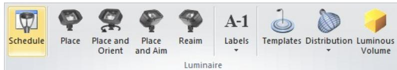
To **Place and Aim** a **Luminaire**, select a **Luminaire Type** from the graphical list. Select the **coordinates** desired for the **Luminaire** location with the mouse, keyboard entry or **Object Snap**. Visual then provides instant feedback by placing the aim point at the mouse **crosshairs** and shows the resultant **Aiming Line** and **Luminaire** orientation as the mouse is moved. Specify the aiming point with the mouse, keyboard, or **Object Snap**.
