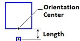
The **Length** of the **Support** is the distance from the *pole* to the edge of the **Symbol**.
