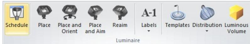
To **Place** a **luminaire**, select a **Luminaire Type** from the graphical list. Select the **coordinates** desired with the mouse, keyboard entry or **Object Snap**.
