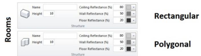
The **Height** of the **Room** or **Structure** must be specified. Note that the **Height** last specified as input for the command will be used as the default (which can of course be changed) upon the next execution of the command; the idea being that heights of **Rooms** and **Structures** will be the same in most cases for a given project.
