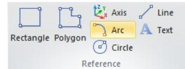
Select the **Arc** start and end *coordinates* by either navigating the mouse *crosshairs* to the appropriate *coordinate* location, entering the *coordinates* numerically at the **Command Line**, or by selecting an object using one of the **Object Snap** methods.
