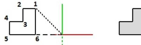
**Solid Polygons** cannot be self-crossing. Visual makes the determination at the completion of the command and provides a message box. All *coordinate* input during the command is lost; therefore careful selection of points should be made.
